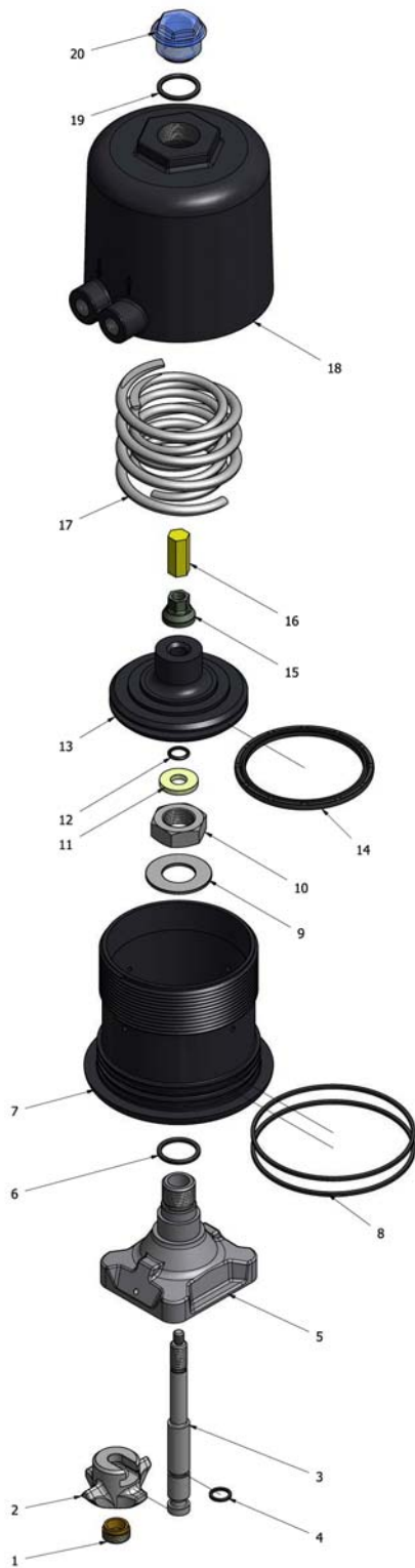
Spring to close exploded view
